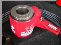
Load Cell Sensor installed on bridle
