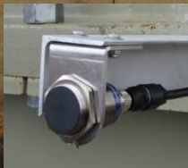
Proximity Sensor mounted behind crank arm
