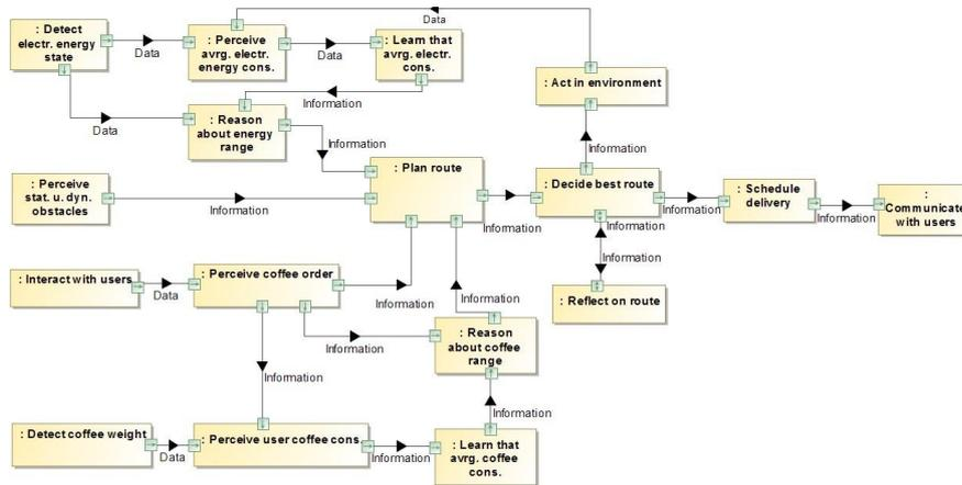
Fig.5: Functional Flow Diagram of the coffee robot waiter
