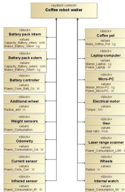
Fig. 8: Hardware modules composition of the coffee robot waiter
